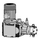
The HYDRO API 675 hydraulic diaphragm metering pumps form an integrated product range with stroke lengths of 15 or 20 mm. Equipped with full-motion drive and automatic bleeding, they therefore cover the capacity range of 7 to 1506 I/h at 100 – 7 bar. They also meet the requirements of API 675.
