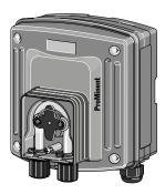
The feed chemical is transported by the rotor squeezing the hose in the direction of flow. This explains why there is no need for valves. The feed chemical is thus handled with care. Typical applications: wherever lower pump pressure is sufficient. For example when metering conditioners in private pools.
