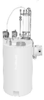
Thousands of steam generators operate in industry. Corrosion in systems equates to idleness, which needs to be prevented. The DULCODOS Ammonia metering system produces a usable solution of 0.1 to 2.5% from the maximum 25% commercial ammonia product. The transfer pump, measuring tank and mixing tank are important for production of the required solution. The beta metering pump meters the solution precisely into the steam system to be protected.
