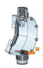
1: Diaphragm rupture sensor
