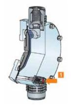
1: Diaphragm rupture sensor
